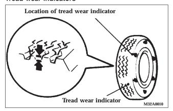
Tread wear indicators are built into the original equipment tires on your vehicle to assist you in determining when your tires have been worn to the point of needing replacement. Many states have laws making tire replacement mandatory at this point.
